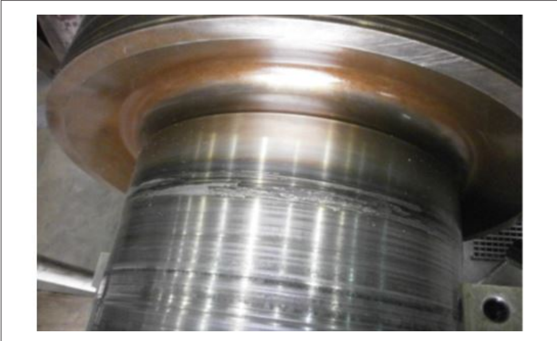
Fig. 4. Rotor journal scoring
